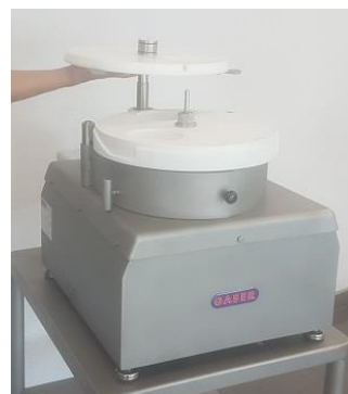
Image 14, Removing tank base
