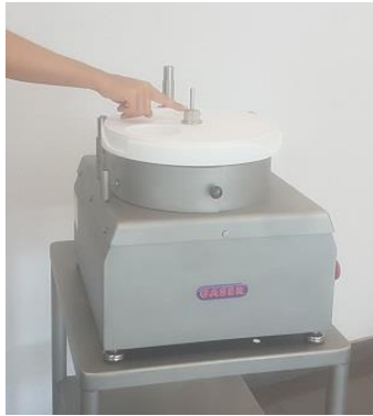
Image 16. Removing former shaft nut
