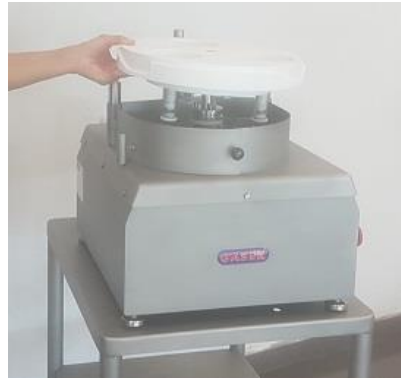
Image 17. Removing former unit
