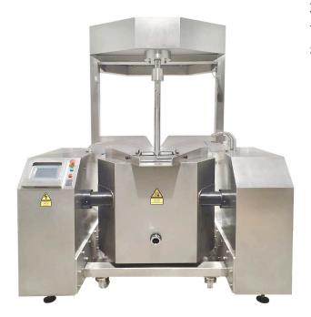
Different models of cooking-kneading kettles from 30 to 300 litres. With variable speed drive and auto lock. Ideal to make all sort of mixtures: croquettes, bolognese and sauces.
